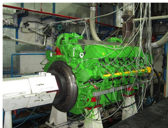
Fig2. D87 dual fuel engine in test cell
